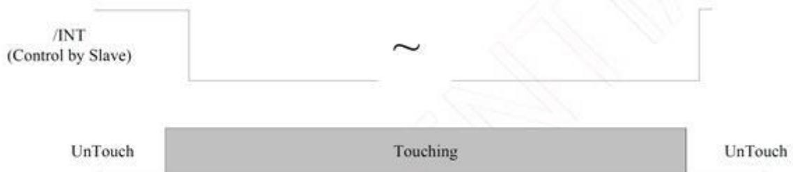
Fig 9: Method 1: \overline{INT} Pin Control Diagram (Finger Touch)
